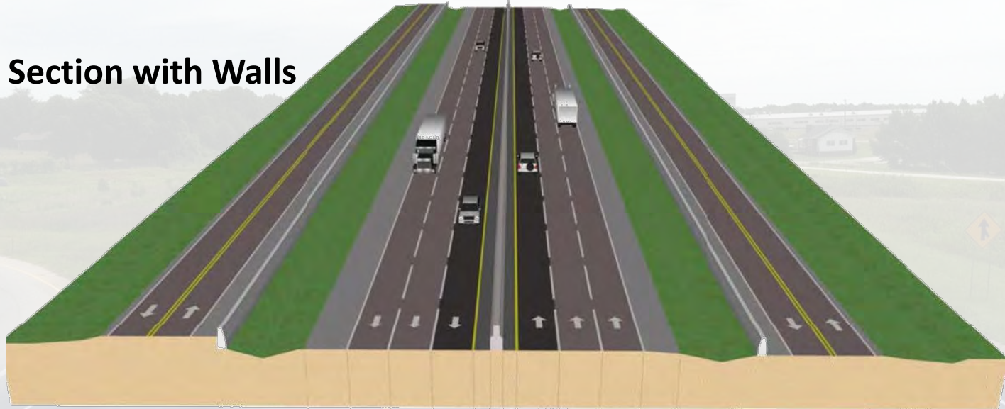
8-Lane Section with Walls to Accommodate for Future Conditions
